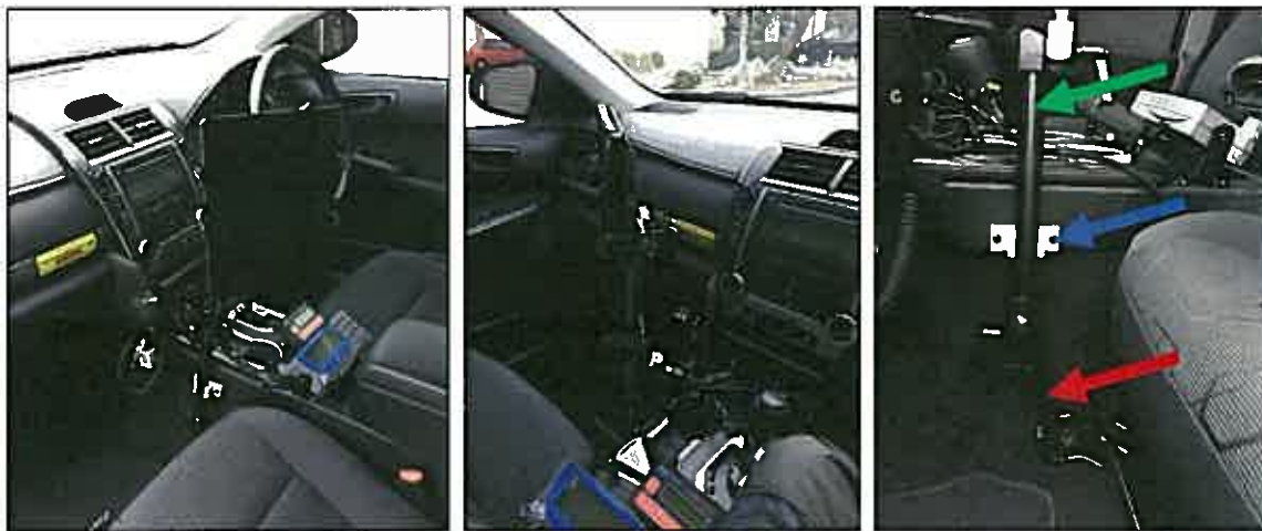
FIGURES 5-6: TABLET HELD IN PLACE BY THE MOUNTING BRACKET ASSEMBLY, FIGURE 7: CLOSE UP VIEW OF FLOOR BRACKET (RED ARROW), PRIMARY BRACKET (GREEN ARROW) AND INTERMEDIATE BRACKET (BLUE ARROW)
